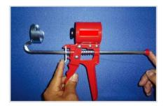
■ Push the red plastic parts while pressing the metal piece above the handle
