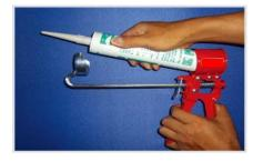
■ Take out the silicone tube and go to the second step for installing of a new one
